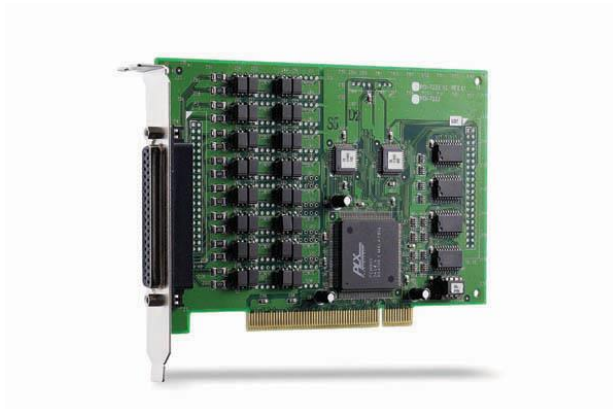
Figure 2-3 Current card used in the old LCU and for which the new LCU code was implemented. This card is installed directly onto the computer motherboard.
