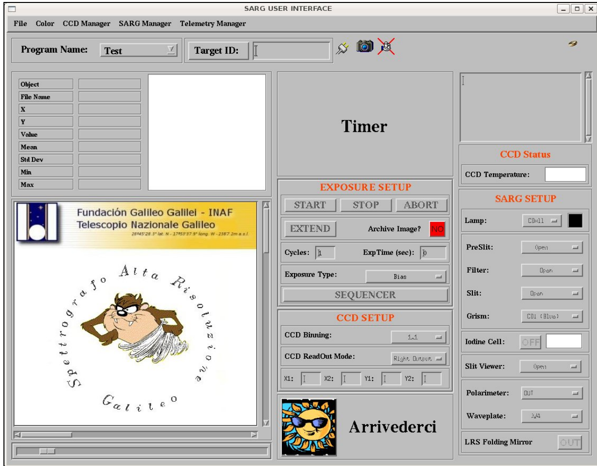
Figure 1. The SARG user interface main panel as it appears when starting an observing session
