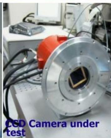
CCD Camera under test
